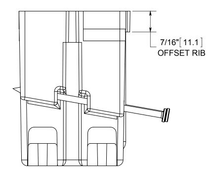
NOTES: 1.) BOX MATERIAL: FIBERGLASS REINFORCED POLYESTER, NAIL MATERIAL: PLATED CARBON STEEL
