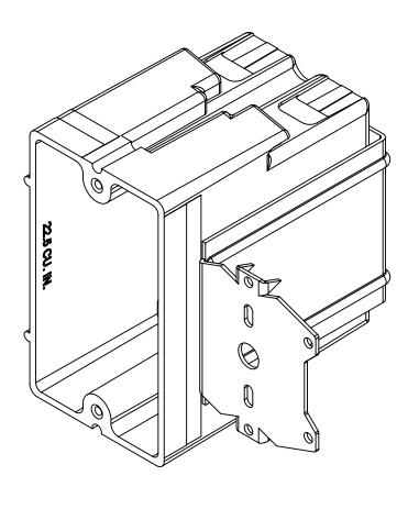
1.) BOX MATERIAL: FIBERGLASS REINFORCED POLYESTER, BRACKET MATERIAL: GALVANIZED
