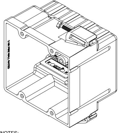
1.) BOX MATERIAL: FIBERGLASS REINFORCED
