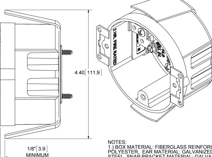
1.) BOX MATERIAL: FIBERGLASS REINFORCED POLYESTER, EAR MATERIAL: GALVANIZED STEEL, SNAP BRACKET MATERIAL: GALVANIZED STEEL, SNAP BRACKET SCREW MATERIAL: ZINC PLATED STEEL, GROUND STRAP MATERIAL: GALVANIZED STEEL, GROUND STRAP MOUNTING SCREW MATERIAL: ZINC PLATED STEEL, GROUND SCREW MATERIAL: GREEN ZINC PLATED STEEL, SPEED KLAMP MATERIAL: PVC
