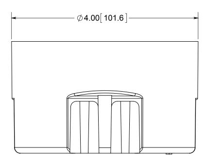
NOTES: 1.) BOX MATERIAL: FIBERGLASS REINFORCED POLYESTER, SPEED KLAMP MATERIAL: PVC 2.) UL LISTED WITH 2 HOUR FIRE RATING FOR WALL AND CEILING 3.) 2 SPEED KLAMPS FACTORY INSTALLED
