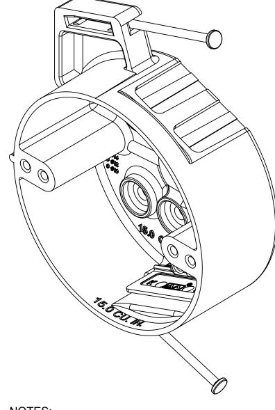
1.) BOX MATERIAL: FIBERGLASS REINFORCED POLYESTER, NAIL MATERIAL: PLATED CARBON STEEL, SPEED KLAMP MATERIAL: PVC
