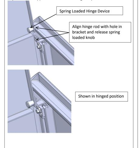
Step 4. Close Swing Out Panel and verify Latch Side Bracket positions. Some slight adjustment may be needed to get final position of the Swing Out Panel exactly where desired.
