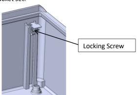
Step 3. Assemble the Swing Out Panel assembly onto the Hinge Side Brackets. Pull the spring loaded hinge device and align the hinge rod with the hole on the Hinge Side Bracket. Release the spring loaded hinge device to engage the hinge rod in the bracket. Repeat for the opposite side of the Swing Out panel.
