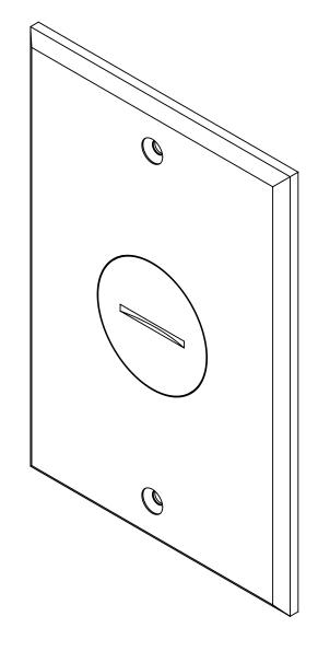
1.) COVER PLATE MATERIAL: NICKLE PLATED BRASS, COVER PLATE MOUNTING SCREW MATERIAL: BRASS, GASKET MATERIALS: POLYURETHANE FOAM, O-RING MATERIAL: SILICONE 2.) WHEN USED WITH FB-5N FLOOR BOX IT IS UL LISTED, FLOOR BOX MEETS UL514C SCRUB WATER **EXCLUSION TEST**
