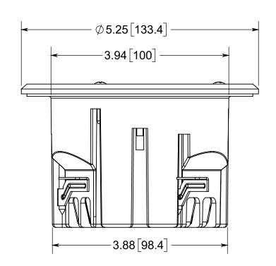
1.) BOX MATERIAL: POLYCARBONATE, COVER PLATE MATERIAL: DARK BRONZE PLATED BRASS, COVER PLATE MOUNTING SCREW MATERIALS: DARK BRONZE PLATED BRASS, DEVICE SCREW MATERIALS: ZINC PLATED STEEL, FLANGE MOUNTING SCREW MATERIAL: BLACK PHOSPHATE COATED STEEL WING MATERIAL: ZINC PLATED STEEL, GROUND PLATE MATERIAL: ZINC PLATED STEEL, GASKET MATERIALS: POLYURETHANE FOAM, O-RING MATERIAL: SILICONE 2.) UL LISTED, FLOOR BOX MEETS UL514C SCRUB WATER EXCLUSION TEST
