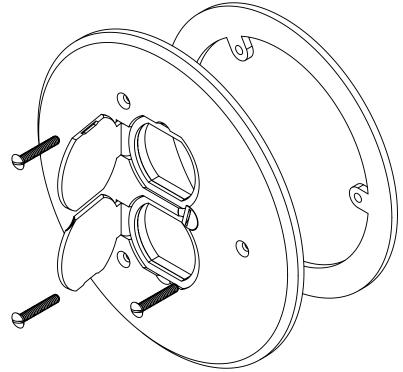
NOTES: 1.) COVER PLATE MATERIAL: BRASS, COVER PLATE MOUNTING SCREW MATERIAL: BRASS, GASKET MATERIALS: POLYURETHANE FOAM, O-RING MATERIAL: SILICONE 2.) WHEN USED WITH FB-4 FLOOR BOX IT IS UL LISTED, FLOOR BOX MEETS UL514C SCRUB WATER EXCLUSION TEST
