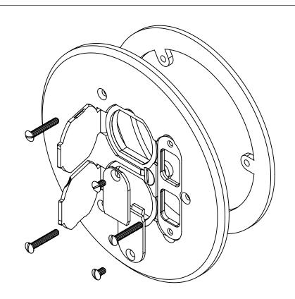
1.) COVER PLATE MATERIAL: NICKLE PLATED BRASS, COVER PLATE MOUNTING SCREW MATERIAL: NICKLE PLATED BRASS, GASKET MATERIALS: POLYURETHANE FOAM, O-RING MATERIAL: SILICONE
