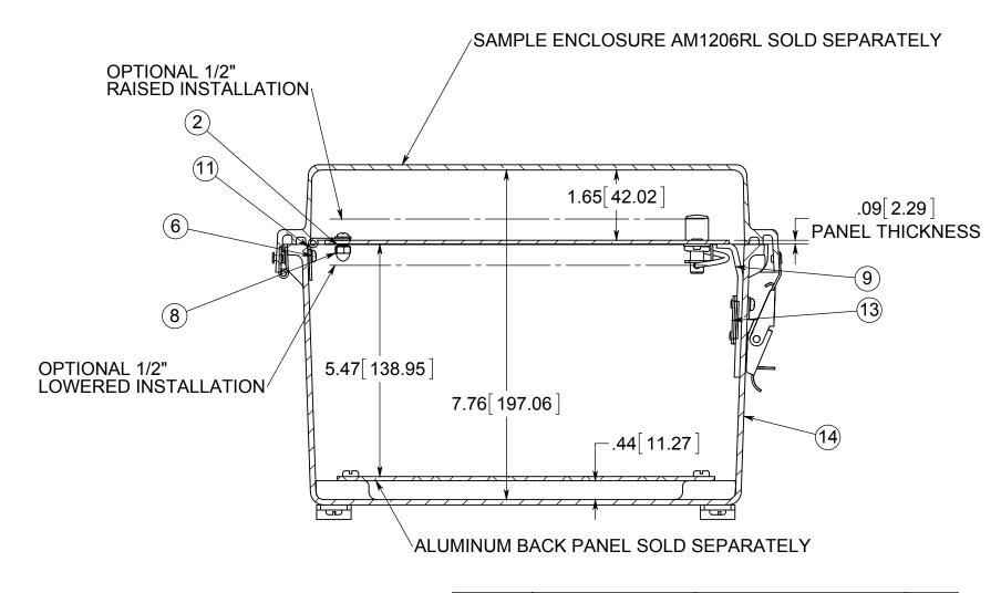
NOT ALL PARTS OF THE HFP ASSEMBLY KIT ARE SHOWN, ONLY THE PARTS USED IN THE FLUSH INSTALLATION OF THE PANEL.
