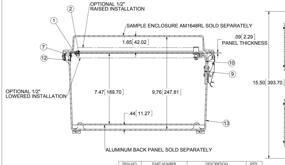
NOT ALL PARTS OF THE HFP ASSEMBLY KIT ARE SHOWN, ONLY THE PARTS USED IN THE FLUSH INSTALLATION OF THE PANEL. FOLLOW INSTALLATION INSTRUCTIONS INCLUDED IN THE KIT FOR THE OPTIONAL PANEL MOUNTING
