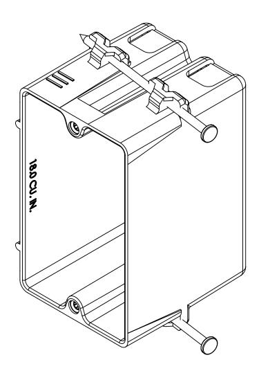
NOTES: 1.) BOX MATERIAL:PVC, NAIL MATERIAL: PLATED CARBON STEEL 2.) UL LISTED WITH 2 HOUR FIRE RATING FOR WALL AND CEILING
