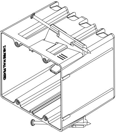
NOTES: 1.) BOX MATERIAL:POLYCARBONATE, NAIL MATERIAL: PLATED CARBON STEEL 2.) UL LISTED WITH 2 HOUR FIRE RATING FOR 3.) ACCEPTS LVP-2 LOW VOLTAGE PARTITION
