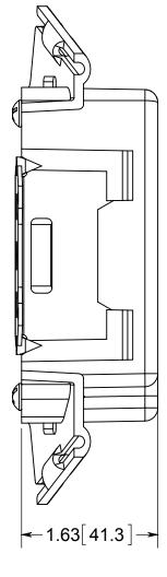
NOTES: 1.) BOX MATERIAL:POLYCARBONATE, MOUNTING BRACKET MATERIAL: GALVANIZED STEEL, SCREW MATERIAL: ZINC PLATED STEEL 2.) UL LISTED WITH 2 HOUR FIRE RATING FOR WALL
