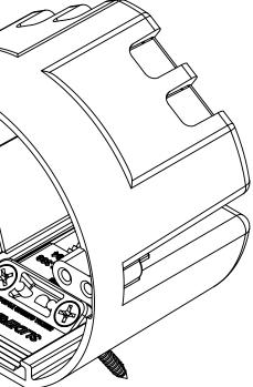
NOTES: 1.) BOX MATERIAL: PC, SLIDER PLATE MATERIAL: PC, SCREW MATERIAL: PLATED CARBON STEEL 2.) UL LISTED WITH 2 HOUR FIRE RATING FOR WALL AND CEILING 3.) TWO 1/2" NM KNOCKOUT 4.) 50-LB FIXTURE RATING
