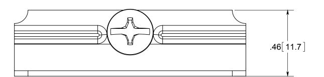
1.) WIRE CLAMP MATERIAL: GALVANIZED STEEL, WIRE CLAMP SCREW MATERIAL: ZINC PLATED STEEL
